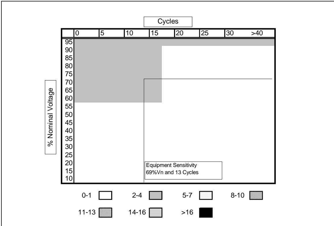
Figure 10 - Facility Voltage Reliability Graph Normalized to a per Year Basis With a 2MVA 660kJ DVR
