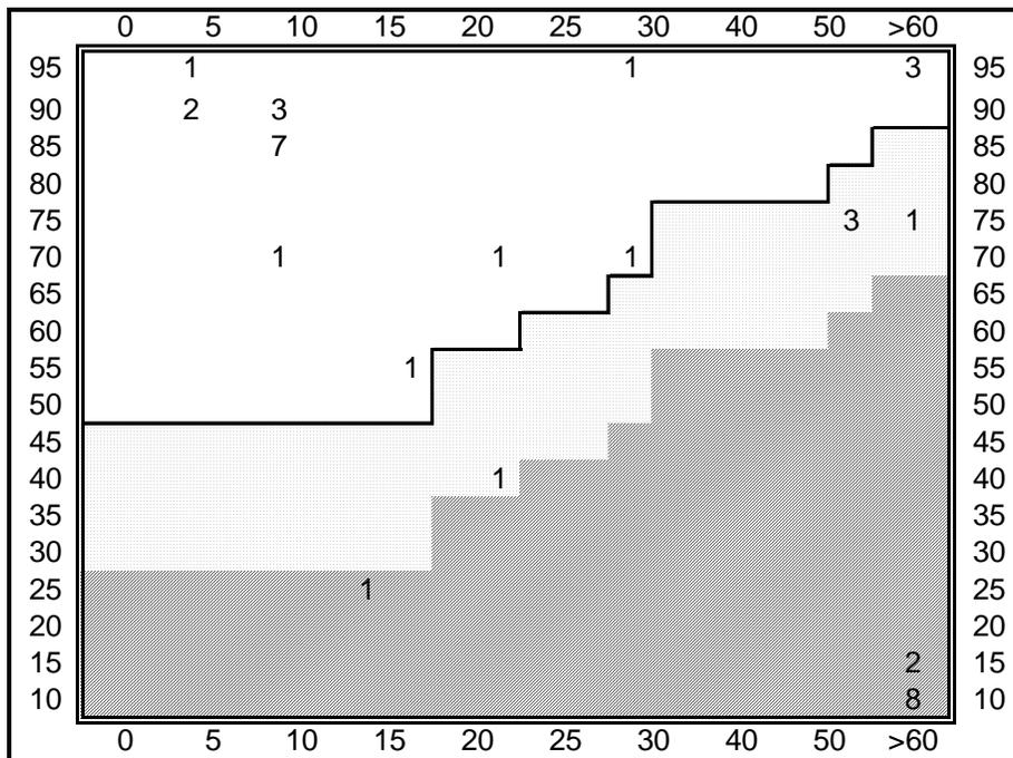
Figure 9 - Facility Events Covered with a 2MVA DVR with 660kJ of Stored Energy And 4.0MVA of Load
