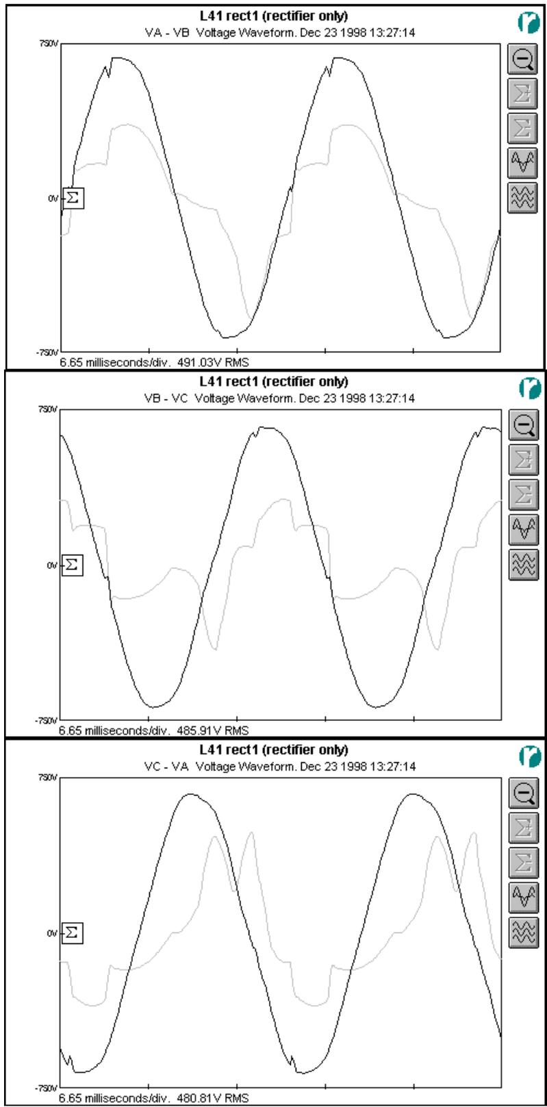
Figure 1 - Rectifier Maximum Recorded Power (Voltage Line to Line)
